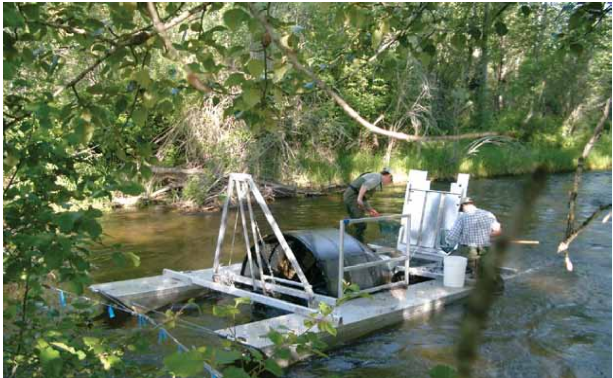
▲ PHOTO 7.7 The rotary screw trap is a very effective long term sampling method. Fish are caught in a cone as the force of the water rotates it. This rotary trap is located on Skalkaho Creek, a tributary to the Bitterroot River in western Montana. (Al Zale, MSU)
