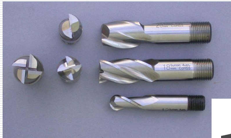
From top: slot , roughing and ball nose end mills
