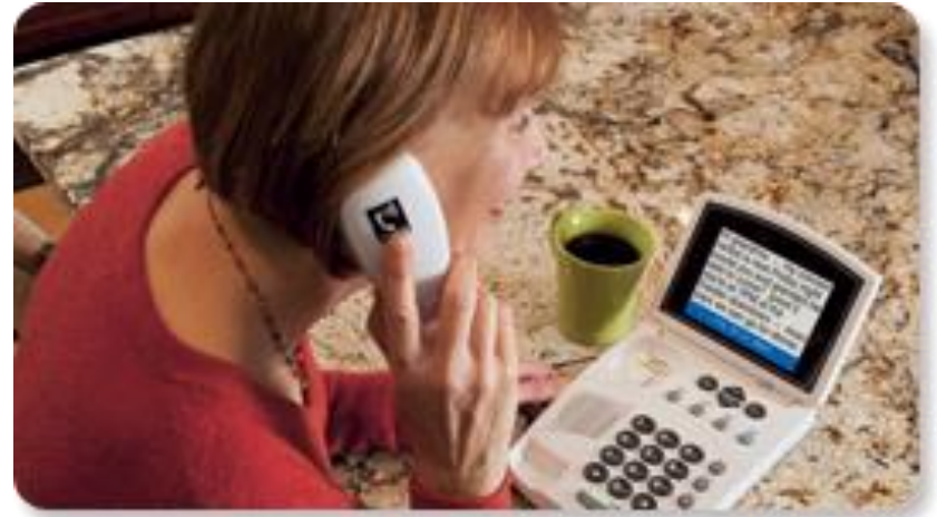
CapTel phone for use by a person who is hard of hearing
