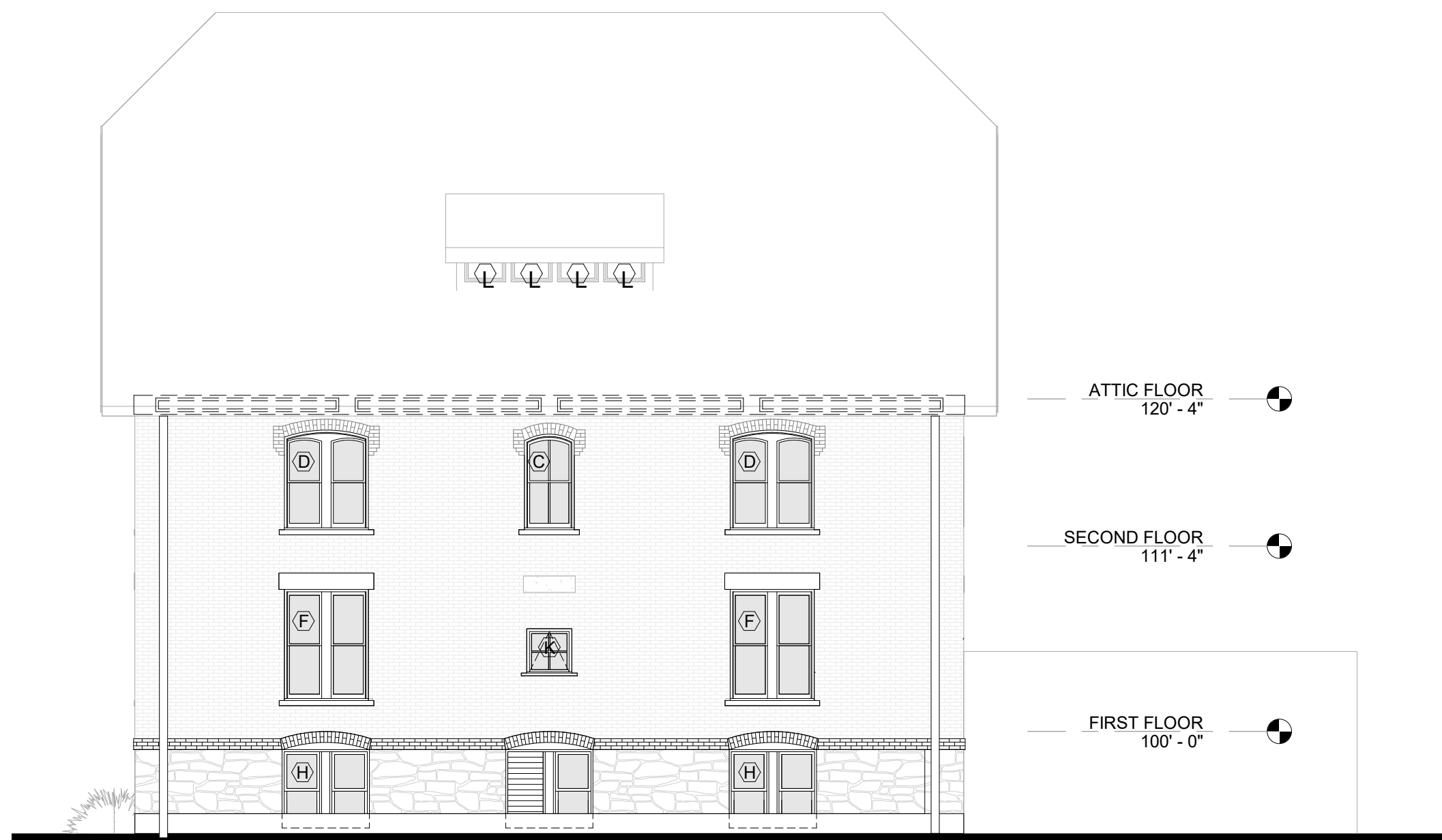
4 SOUTH ELEVATION - WINDOW REPLACEMENT A5.0 1/8" = 1'-0"
