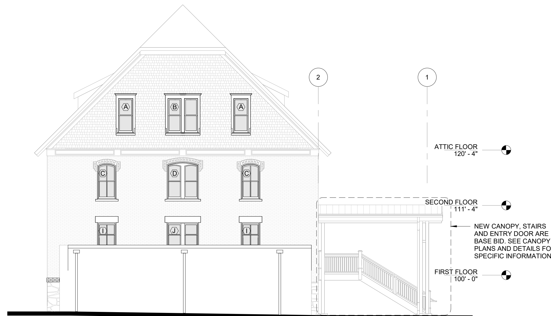
2 EAST ELEVATION - WINDOW REPLACEMENT A5.0 1/8" = 1'-0"
