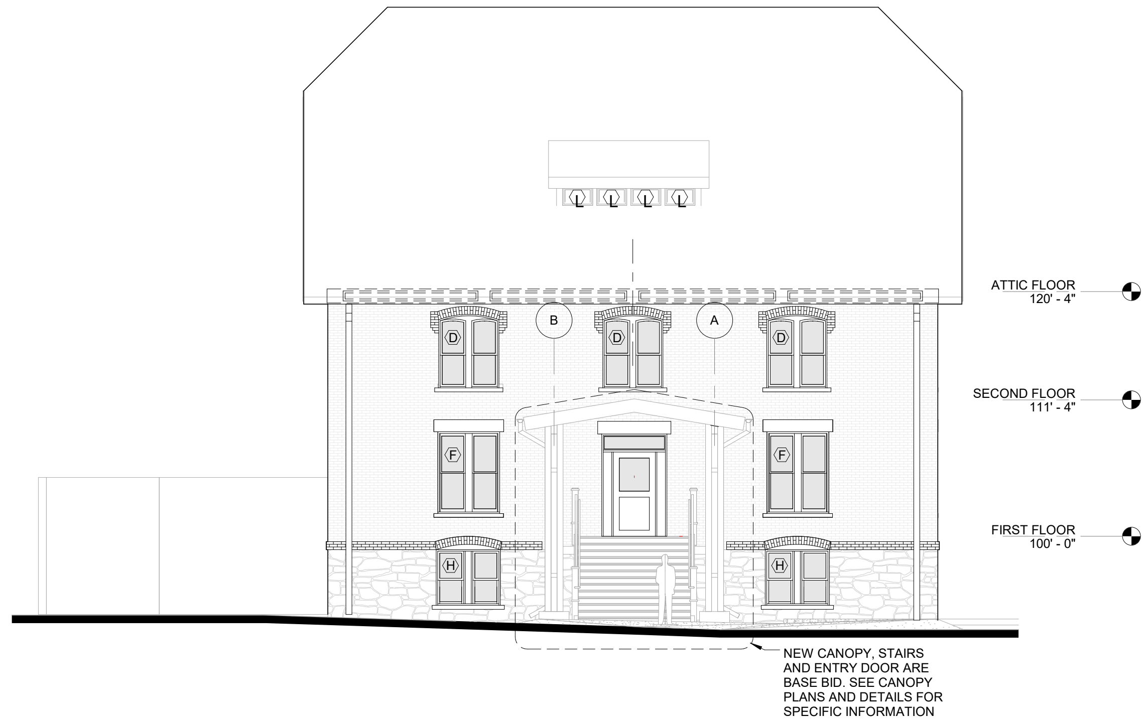
3 NORTH ELEVATION - WINDOW REPLACEMENT A5.0 1/8" = 1'-0"
