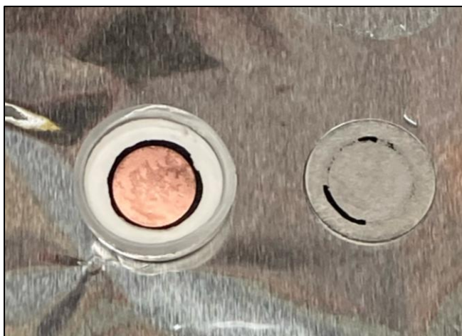
Figure 3. Opened coin cell with ZTC anode after extended cycling and SEI formation.
