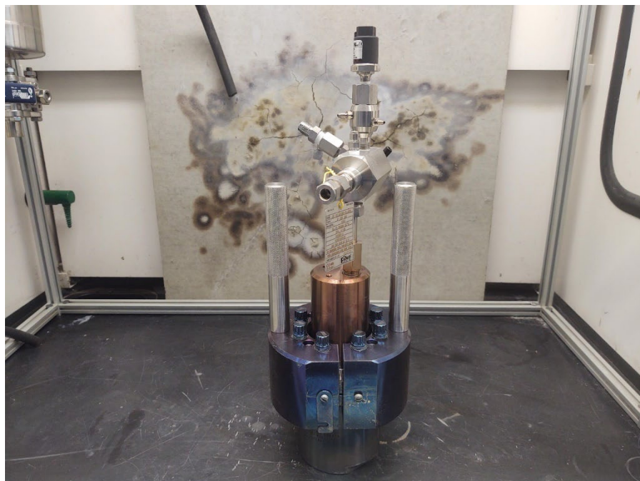
Figure S6. Custom metal reactor removed from the furnace, shown post reaction and prior to opening.
