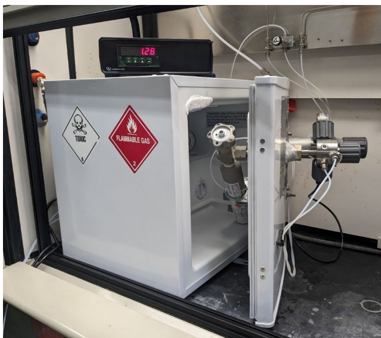
Figure S3. Experimental apparatus for storage and delivery of diborane: lecture bottle containing the B 2 H 6 /H 2 mixture (center) within a freezer held at -20 °C, a purgeable regulator (right), pressure transducer controller (top center), and purge, vent, and delivery gas lines (right and top right) inside a fume hood.
