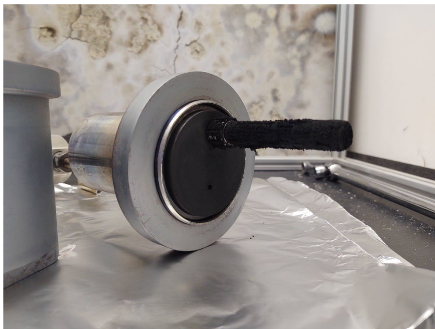
Figure S7. Custom metal reactor head and thermowell, shown post reaction (benzene pyrolysis at 700 °C) and after opening.
