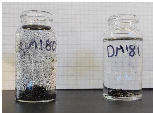
Figure S11. Two solid products generated by the pyrolysis of B 2 C 10 H 14 (NDB) at 800 °C (route IV) can be seen: a suspension of flakes (left) and the remaining mound of the majority solid (right).
