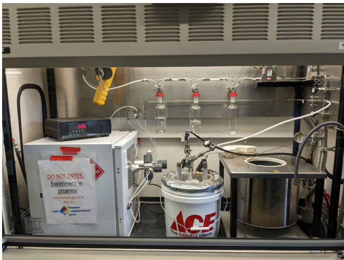
Figure S5. Experimental apparatus for diborane/benzene co-pyrolysis reactions (route II): custom metal reactor (center), furnace (center right), freezer containing the B_2H_6/H_2 mixture (left), purgeable regulator (center left), gas manifold (Teflon and stainless steel), vacuum outlet (right), and abatement system (top center). The reactor is shown submerged in an acetone and dry ice bath at -78\text{ }^\circ\text{C} .
