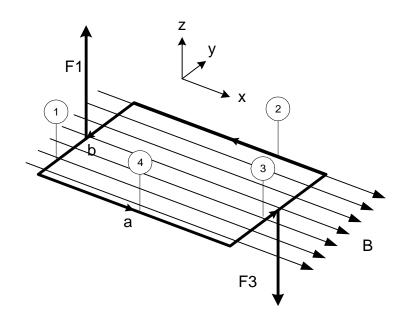
There is no force on leg 2 and leg 4, since the current is parallel to the magnetic field
