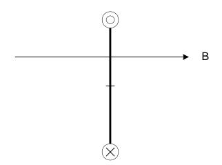
The torque is zero when the B-Field is perpendicular to the plane of the loop.
